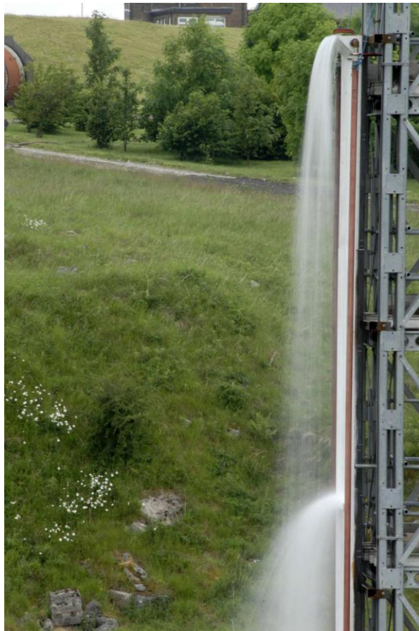
Figure 2 Photo of a vertical section of tank wall showing the liquid spray falling over around 15 metres.
