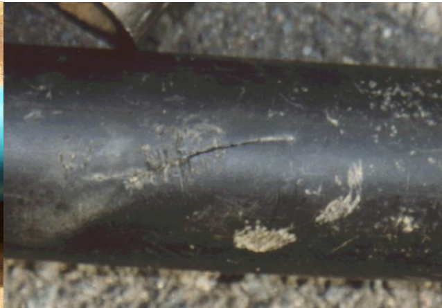
Stage 2 – Slow Crack Growth
