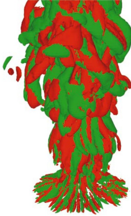
Figure 3 An instantaneous snapshot of the puff cycle from DesJardin et al. [1] showing the finger-like azimuthal instabilities near the base of the plume. The isocontour of streamwise vorticity is shown at \pm 10\% of the peak value.
