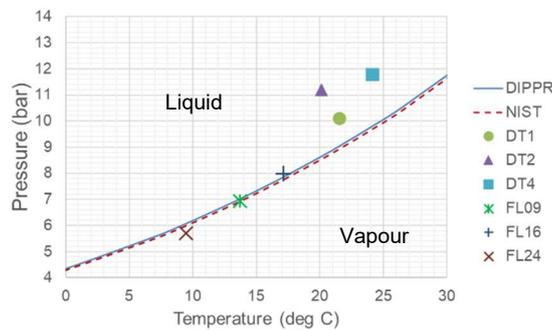
**Figure 1.** Pressure –temperature phase diagram for ammonia. The markers show the phase at the exit conditions for the Desert Tortoise and FLADIS trials.
