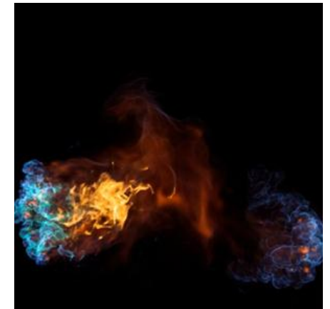
Flame front propagation after ignition by falling droplet
