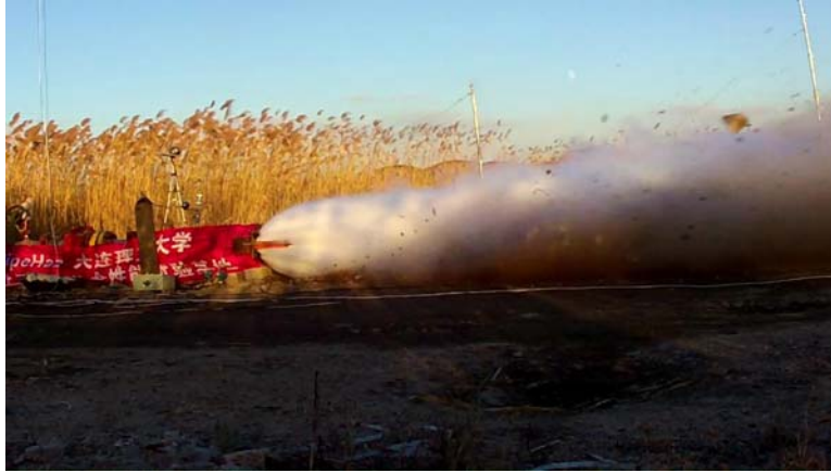
Fig. 13. High speed CO 2 jet following full bore rupture release test from an initial pressure and temperature of 36 bar and 3 °C.
